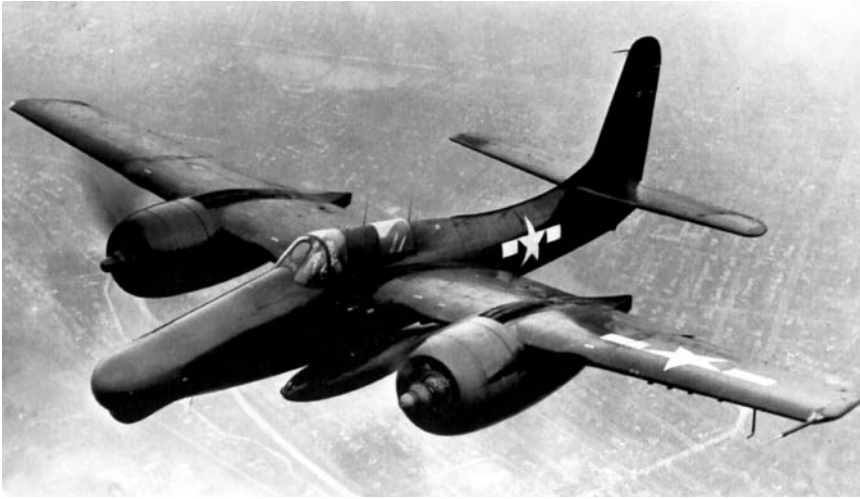
Used as a night fighter during the early years of the war, the two-seat, twin-engine Grumman F7F-3N Tigercat, with its distinctive nose-mounted radar and taller vertical tail, repeatedly proved its capabilities. (Marine Corps Historical Center Photo Collection)
