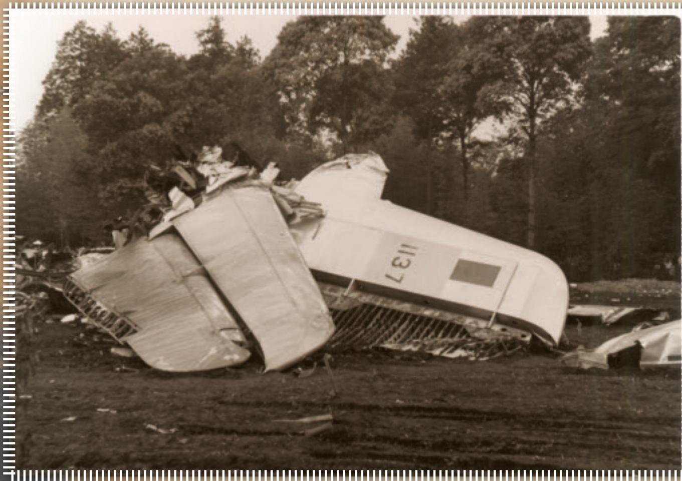
The vertical stabilizer was ripped off C-124 No. 51-137 when the aircraft hit the ground near Tachikawa AB, Japan.
